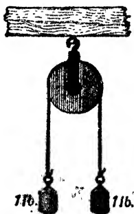
FIG. 95. A common pulley.
